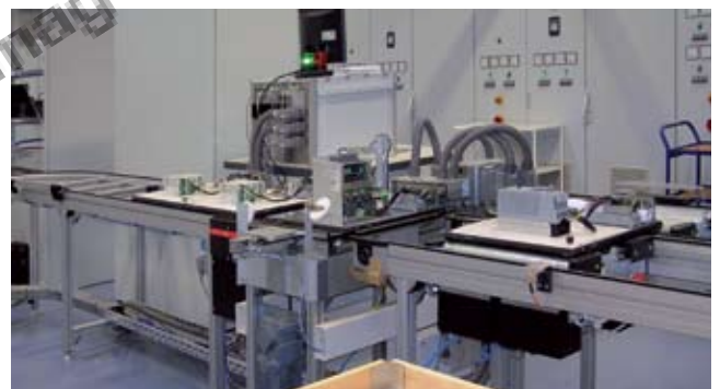
Automatic high voltage testing system
